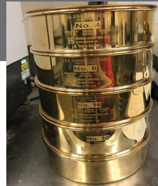
Image 2 – Sieve stack used to determine the RCI. Sieves can be used to assess the level of fines in a grain sample.
